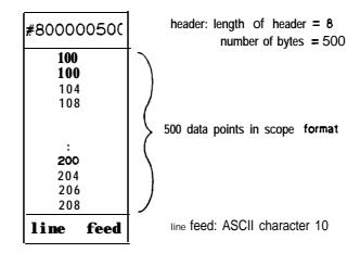
The waveform data inside the oscilloscope can be transferred out in a variety of formats. The data is in a defined block format with a header specifying the length of the block. The block is terminated with a line feed character (ASCII character 10).
