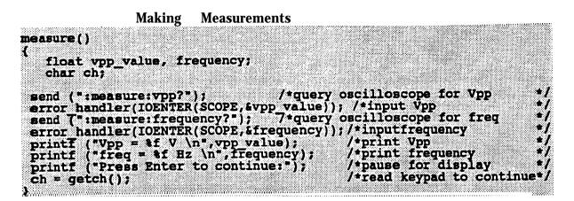
After a digitize command, the signal is displayed on the screen and the acquisition process is stopped. Any of the parametric measurements can be made on this data using either the parametric measurements (such as Vpp, frequency, pwidth) or markers (such as VTIME, TVOLT, **ESTART)**. All measurements use the IEEE standard for making measurements.
